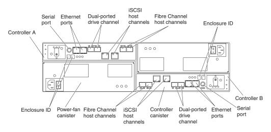
Figure 4. Back view; controllers with two standard Fibre Channel host expansion channels and two optional iSCSI host expansion channels
